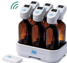
RESPIROMETRIC Sensor System BOD
