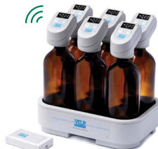
RESPIROMETRIC Sensor System BOD
