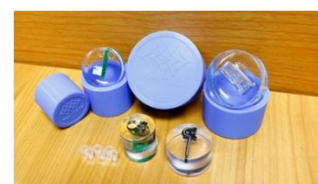
Sample after cold mounting
