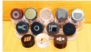
Sample after grinding &amp; polishing
