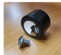
Sample after grinding & polishing
