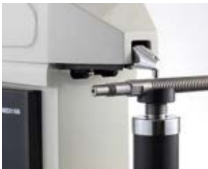
Screw lead hardness test
