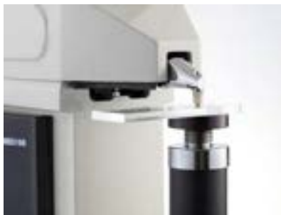
Plexiglass plate plastic Rockwell HRMW test
