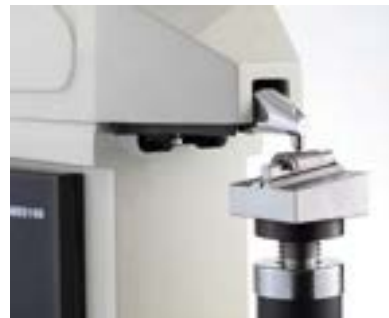
Hardness test of anchor clip
