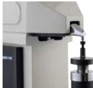
Surface hardness test of pin shaft
