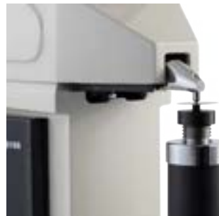
Use diamond specimen support to test HR30Tsm and HR15Tsm of thin tin plate
