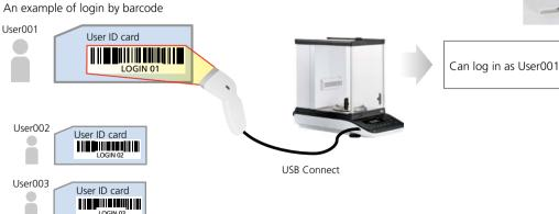
An ID and password are needed to log in to the AP series if protected access is activated. With the barcode, an operator can log in by scanning the barcode instead of inputting an ID and password.
