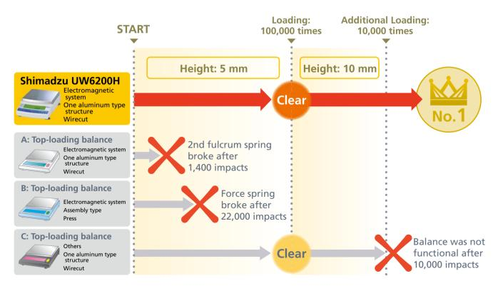
The results of this impact resistance test prove Shimadzu UW/UX series balances with UniBloc technology are the toughest. Put Shimadzu balances in your lab and experience UniBloc power.
