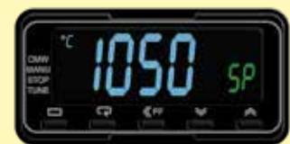
Example of an over-temperature limiter
