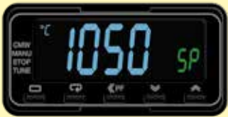
Example of an over-temperature limiter
