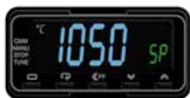
Example of an over-temperature limiter
