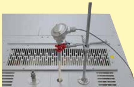
Thermocouple port in the ceiling with tripod
