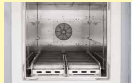
Roller conveyor in furnace chamber
