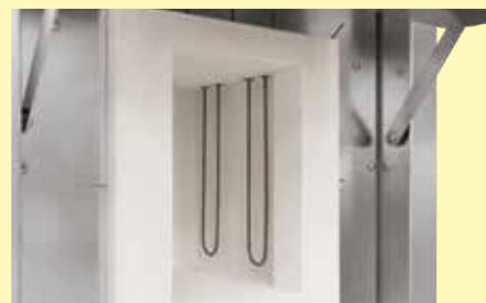
High-quality molybdenum disilicide heating elements
