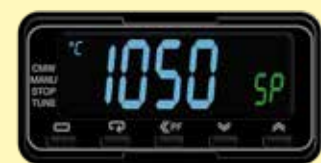
Example of over-temperature limiter
