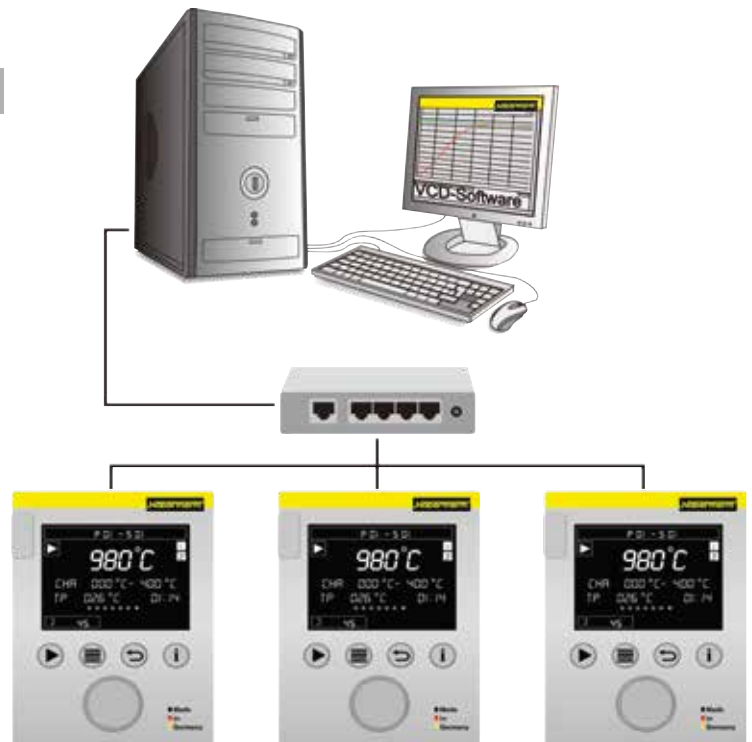
Example lay-out with 3 furnaces
