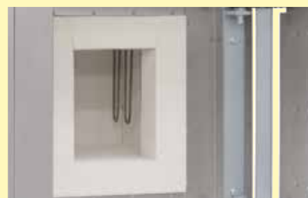
Light-weight refractory bricks and heating elements made from molybdenum disilicide
