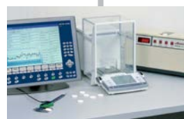
Testplace module with weighing station, tablet tester and dimension measurement
