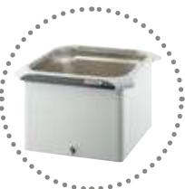
**Stainless steel bath tanks up to +150 °C, insulated**
