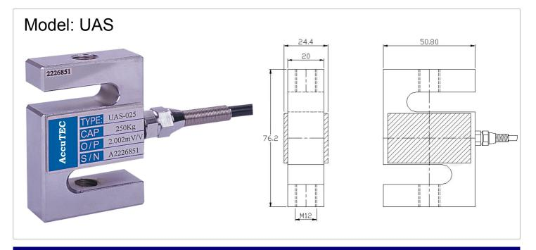
AccuTEC load cells are designed to meet the most stringent accuracy requirements. UAS universal load cells are available in the capacities 250 Kg to 750 Kg. They offer total alloy steel construction and complete hermetic sealing,making them suitable for use in the toughest industrial environments.
